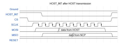
If HOST\_INT is asserted before HOST starts its transmission, TX/TX conflict resolution takes place. NCP will receive HOST packet, because NCP I/O continues receiving until CS line is deactivated, check received packet, recognize conflict, pass RX packet to LL algorithm and retransmit its failed TX packet immediately.
