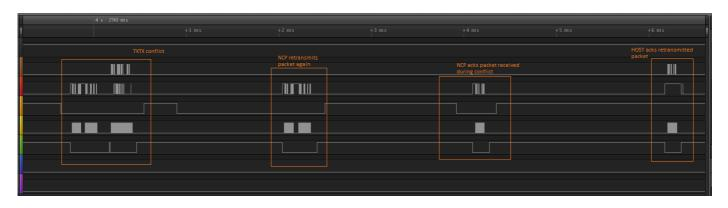
For normal cases, diagrams from chapter 3.3 can be referred to, when NCP wants to send something it asserts HOST\_INT pin and waits for SPI clocks to start sending data. Host handles an interruption from HOST\_INT pin and generates SPI signals to read data from NCP.
