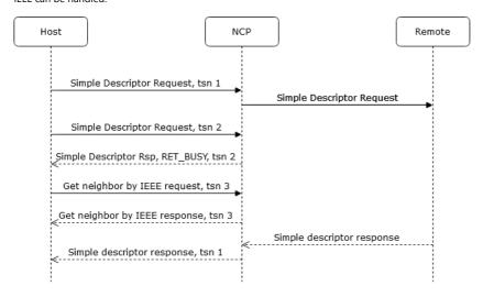
Timeout referred below means maximum time for processing request inside stack including communication with remote node if required, but without HOST-NCP transport overhead, which can be introduced by rate, Host/NCP latency and similar delays.
